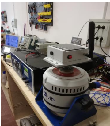
Figure 1 : Experimental set-up for testing WiseSensing frequency resolution in noisy environments
