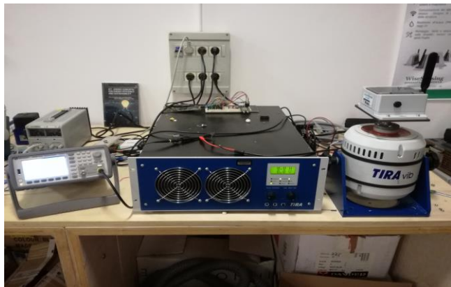
Figure 1 : Experimental set-up for testing WiseSensing frequency resolution in noisy environments
